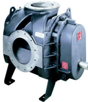
**1. Tri-lobe impellers** operate with less pulsation and lower vibration—less shock is transmitted to bearings. You also get improved volumetric efficiency and up to 10% greater flow.
